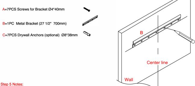
Drill holes for the screws in the positions you have marked with the pencil. Drill the holes' deepth no less than 1 1/2", insert "C" to the holes by using hammer if wall studs are not in the correct positions.
